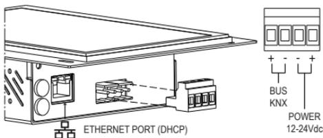
Use only supplied connector to connect with the **BUS**, respect polarity.
